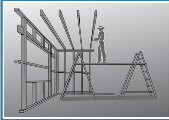
FIGURE 12 Installing ceiling or upper level floor joists
