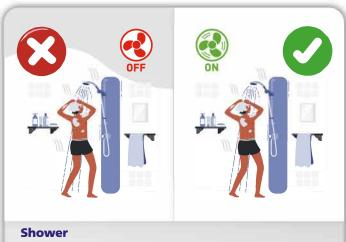
All that surface water and steam in the bathroom has to go somewhere. Always switch on the fan when showering and leave it on until the steam inside the bathroom has gone. Consider using a fan with a humidity sensor that automatically switches on and off depending on the amount of moisture in the air, or simply open a door and window. Natural ventilation enables the extraction fan to achieve optimal performance. Water vapour: 1.5 litres per day
