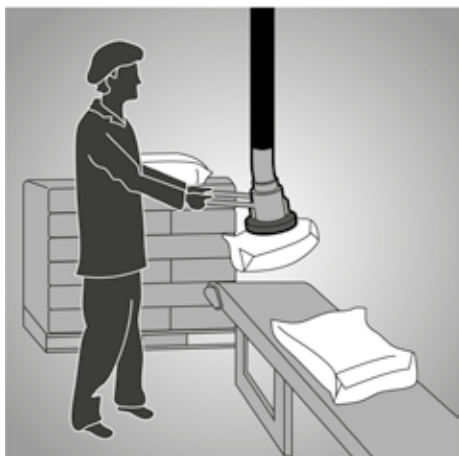
Figure 45 - A vacuum lifter reduces the need to bend and lift when palletising
