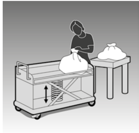
Figure 46 - A self-adjusting base in the laundry tub reduces the need for bending and twisting during unloading
