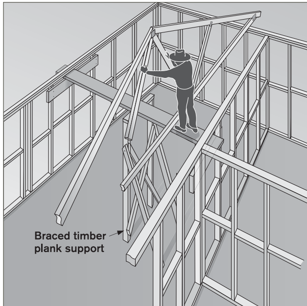
Figure 19 Truss erection – internal support (fall protection for persons working at the perimeter has been omitted for clarity).
