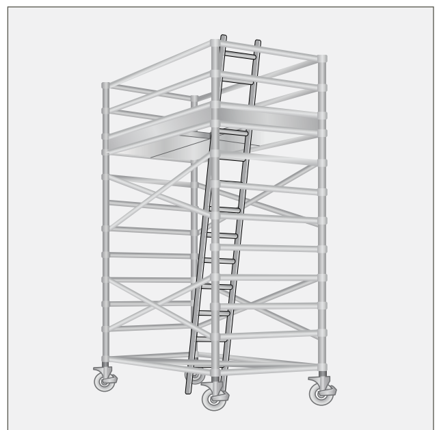
Figure 5 Mobile scaffold with an access ladder and a trapdoor to provide the largest possible hazard-free working platform.
