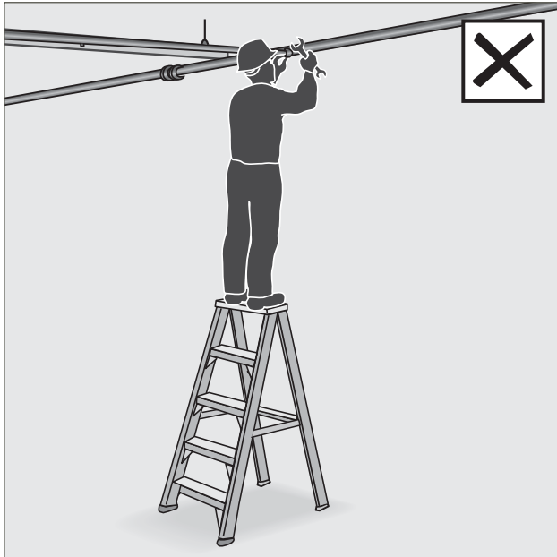
Figure 24 Hazard – standing above second topmost tread of stepladder.
