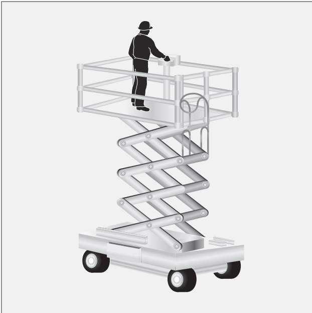
Figure 10 An example of a scissor-lift elevating work platform. As with boom-type platforms, people should not climb onto or off the platform when it is in an elevated position. A safety harness system is not required on this item of plant unless advised by the manufacturer or indicated in the risk assessment and a suitable anchor point is provided.
