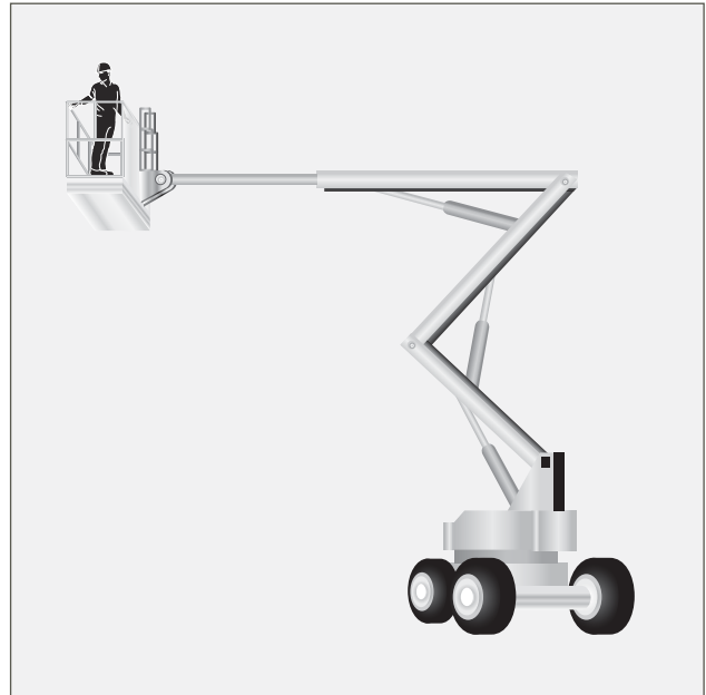
Figure 9 An example of a boom-type elevating work platform. The safety harness and lanyard assembly are not shown for purposes of clarity. The lanyard needs to be as short as possible and be attached directly to the designated anchor point, not to the handrail.
