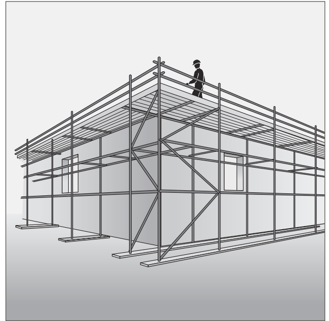
Figure 4 Perimeter scaffold with a fully decked working platform, guardrails and toeboard.
