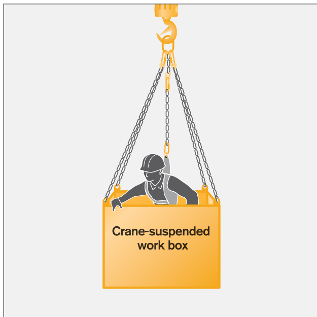
Figure 12 An example of a crane-suspended work box.
