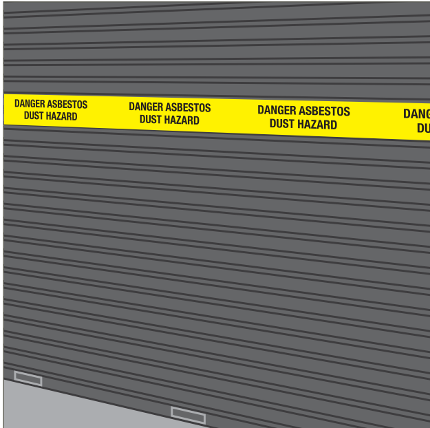
Figure 4: Barrier formed using tape (appropriate for small non-friable removal jobs or as part of system using other barriers such as hoarding).
