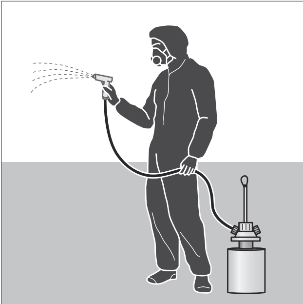
Figure 6: Spray using a low-pressure sprayer.
