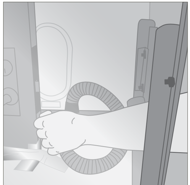
Figure 6: Side view showing the operator using the vacuum hose to 'shadow vac' below the screw as it is unscrewed from the lock housing.
