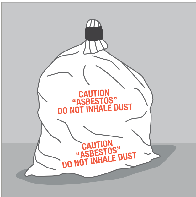
Figure 10: An asbestos waste bag with appropriate warnings.
